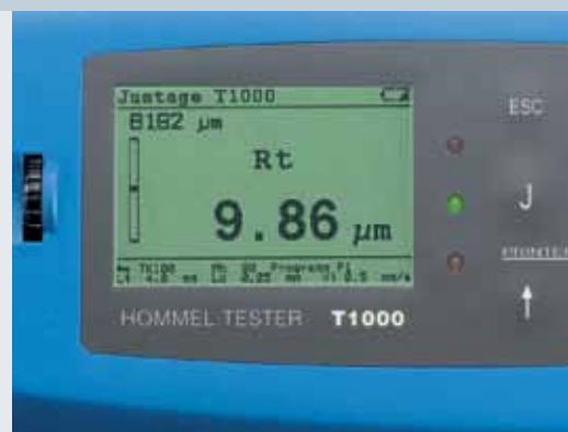
Large graphical display, knurled wheel and function keys, tolerance light
